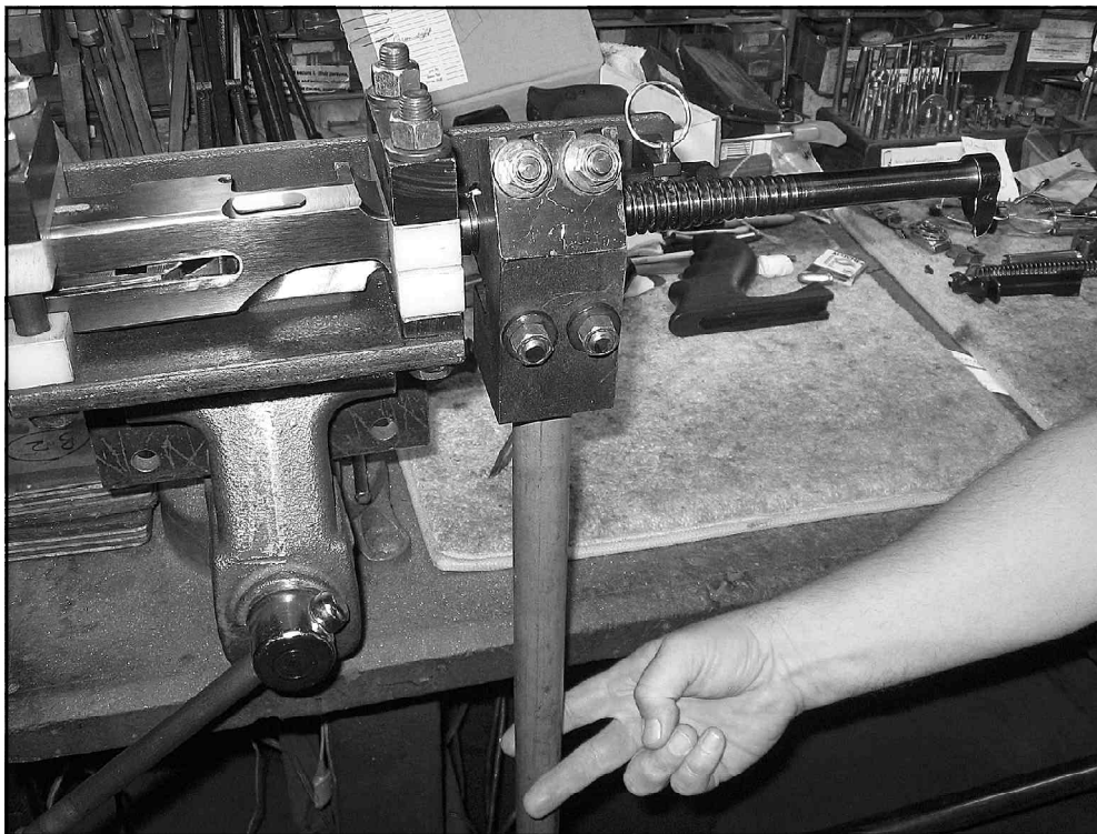
Left: Phoenix gunsmith Nelson Ford using special tooling to remove the barrel of a 1921 Colt Thompson.
