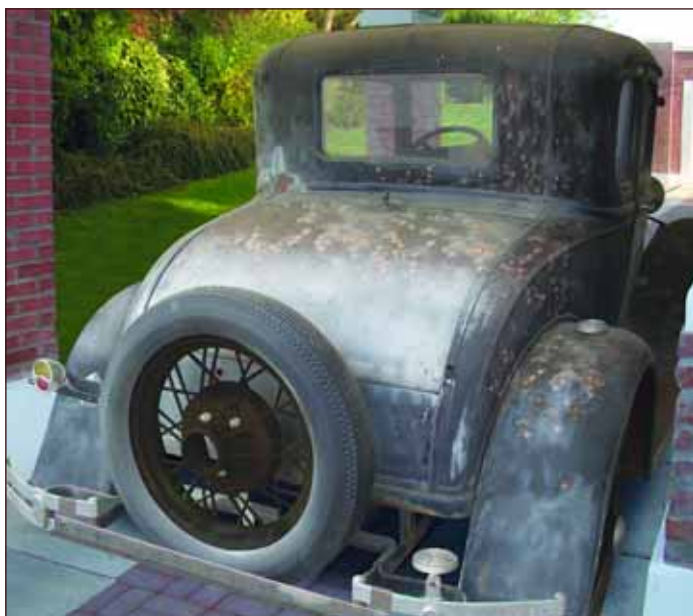
Prior to restoration, the Coupe was documented photographically. This view clearly shows the broken rear window, the bullet hole and rear bumper cross bar. All items that appear in the period
