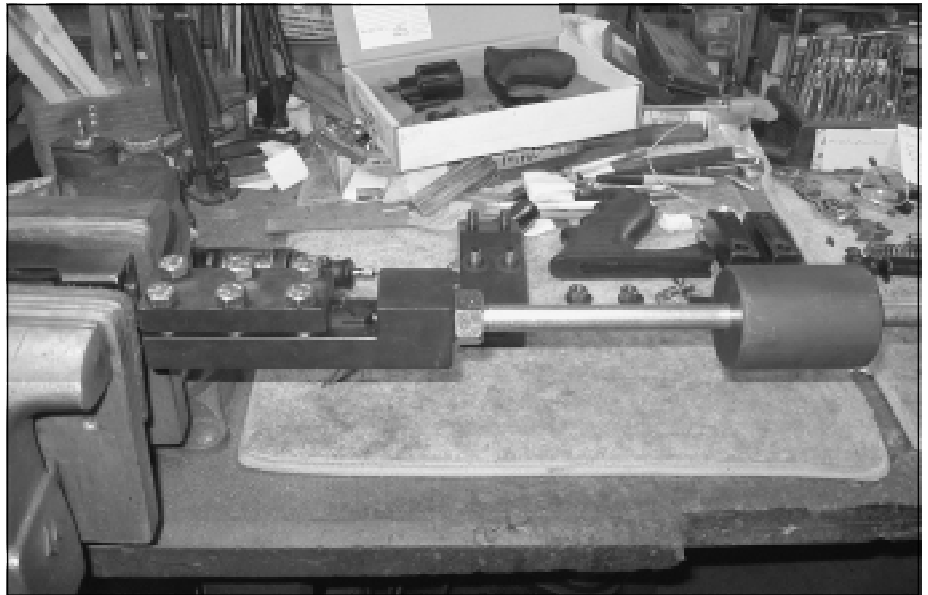
Above: The Richardson Grip-Mount Puller, shown in position here, is essentially a type of slide hammer.
